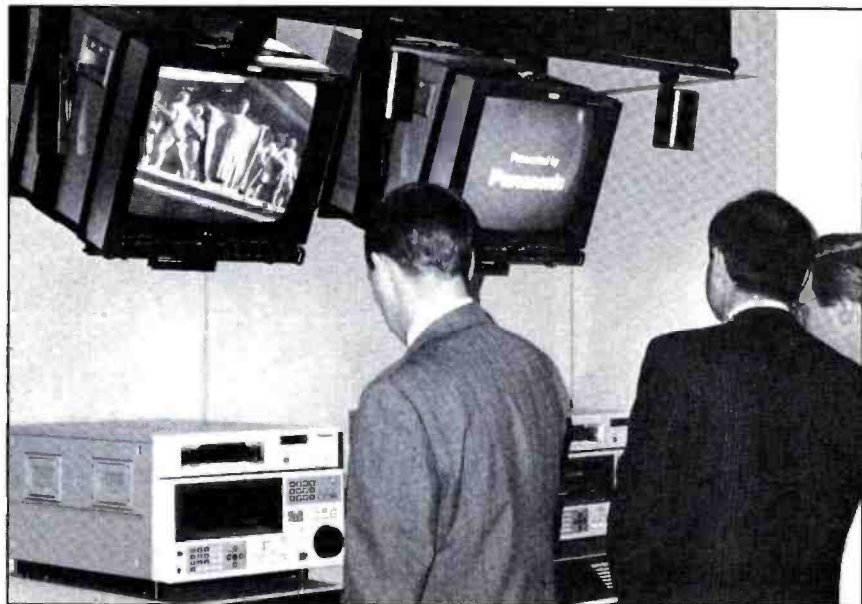
A display of half-inch digital VTR's at the Society of Motion Picture and Television Engineers exhibition last fall. The format is being proposed as the alternative to D-2 for digital TV acquisition.
